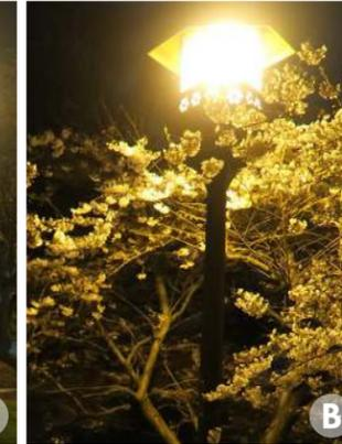
Correlated Color Temperature (CCT)\* of light sources throughout the neighborhood is typically 3500K in the case of the current pedestrian pole light, 4000K for roadway lights, and 2200K for High Pressure Sodium floodlights. As such, the variety of sources create a patchwork experience of lighting color at night. (A)
