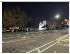
Under freeway, Jackson bus stop The bus stop sign on Jackson is mounted on a pedestrian streetlight that is not working. Under the freeway, there are multiple flood lights which are supposed to provide light to the sidewalk. None of the light fixtures in the area are working. The light from the roadway fixtures outside of the freeway area slightly help to improve the light level.
