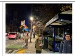
12<sup>th</sup> and Weller Bus Stop – East Side Unlike the west side, the bus stop on the East side of the street and shelter is poorly lit. There are no nearby pedestrian pole fixtures and overgrown branches around the shelter block light from nearby cobra head fixtures. The shelter is also devoid of an integrated downlight.
