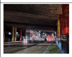
Jackson and Maynard Valley This stop and shelter are near a King fixture which is also the main light source for it. The fixture is likely located too close to the bus shelter which casts a dark shadow over the shelter. The storefront around it is unlit. The light fixture inside the shelter is also not working. The location does not feel safe due to loitering pedestrians.
